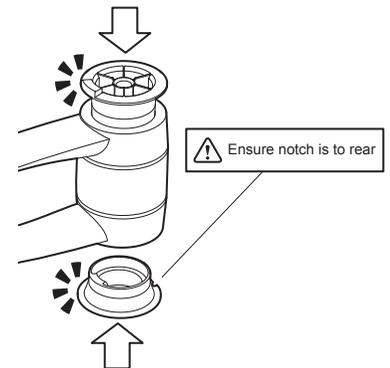
**6** Add arm to the bracket and insert spacer screw
