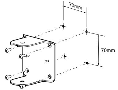
**!** Bolts should be Xmm in diameter and suitable for 12kg (26.5lbs) min
