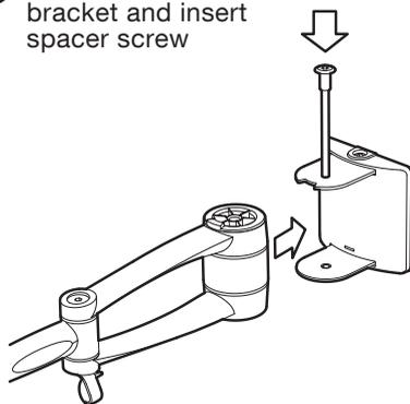
**7** Tighten spacer screw
